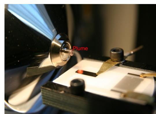
The SAWN-generated ions come directly from a planar surface simplifying the sample preparation process. Also, as an ambient ionization method, SAWN can limit uncontrolled fragmentation of the precursor ions. SAWN can be operated in continuous mode as in ESI or pulsed mode like MALDI depending on the sample introduction.
