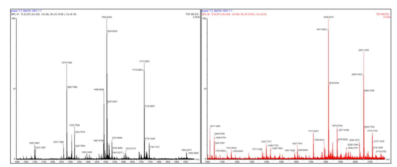
Synthetic mono- and diphosphoryl lipid A were obtained commercially and analyzed by SAWN. Approximately 50 nmol sample in 2:1 chloroform:methanol were deposited onto SAWN chip. Spectra were acquired in negative mode using Waters Synapt G2S™ HD MS.
